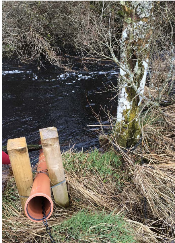
Figure 10: Constant water quality monitoring at Waterside (Grid reference: 228993 572210). Exo1 sonde is housed in a pipe and secured to the river bank to remain in situ for several months
